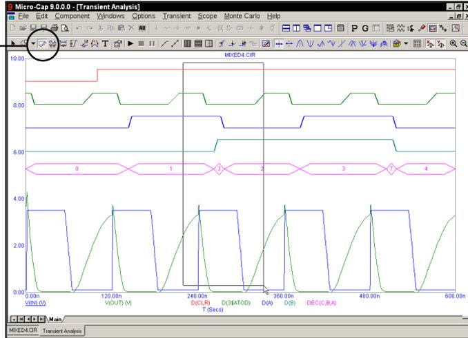
Figure 2-4 Using the mouse to magnify a waveform
