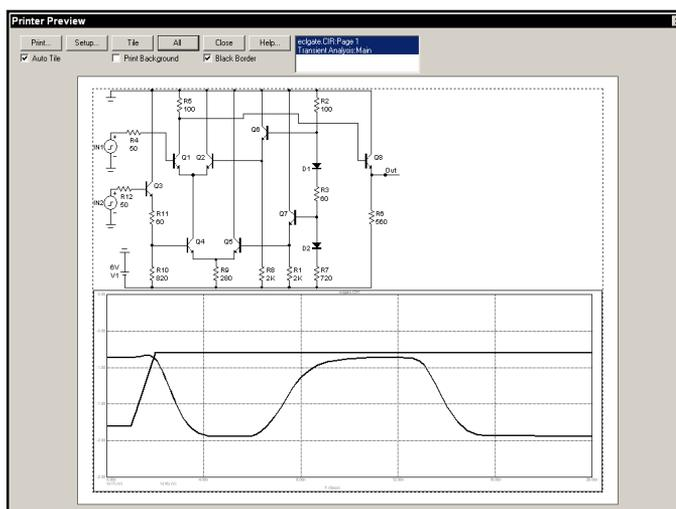
**Figure 13-5 Adding the schematic to the analysis plot**
