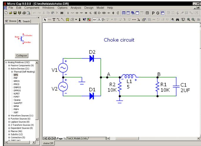
Figure 7-1 The CHOKE circuit
