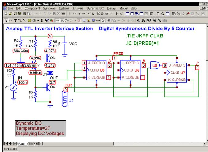
Figure 2-6 Operating point node voltages and states
