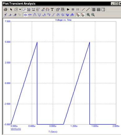
**Figure 3-4 Characteristic plot of the source with TF=0n**
