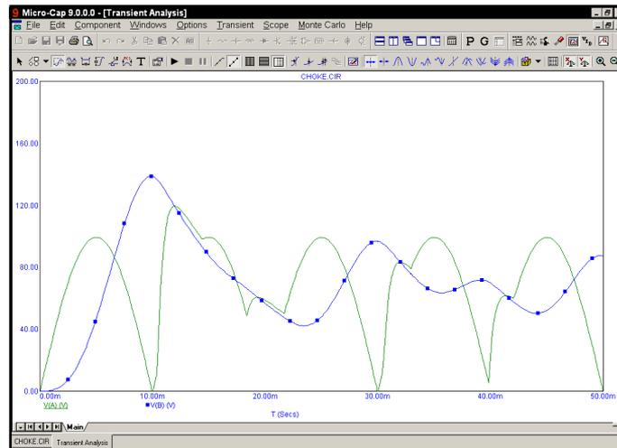
Figure 7-2 Transient analysis of the CHOKE circuit
