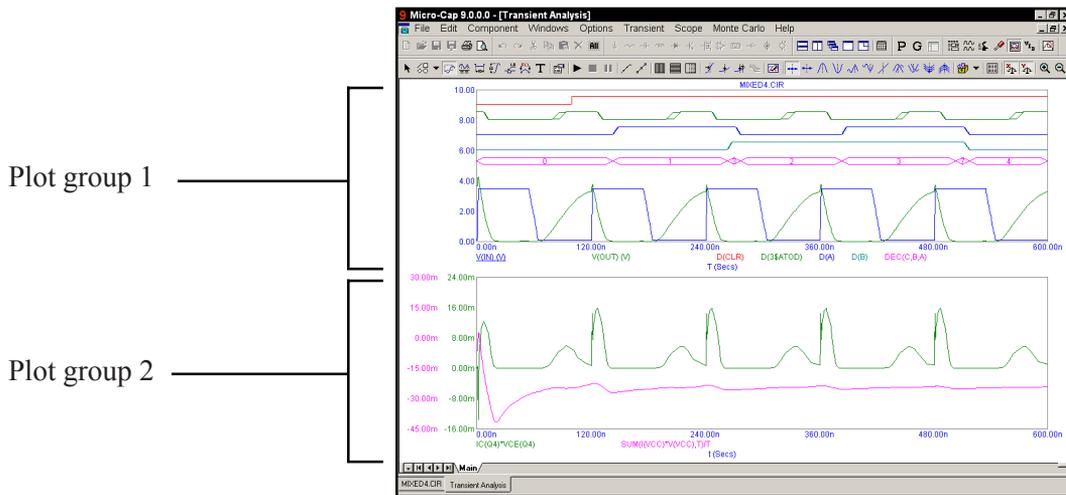
**Figure 4-3 Transient analysis with two plot groups**
