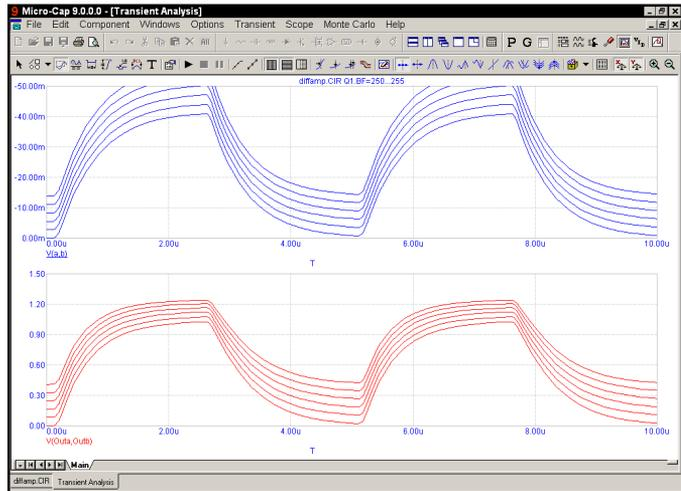
**Figure 9-3 Stepping BF in a single transistor**
