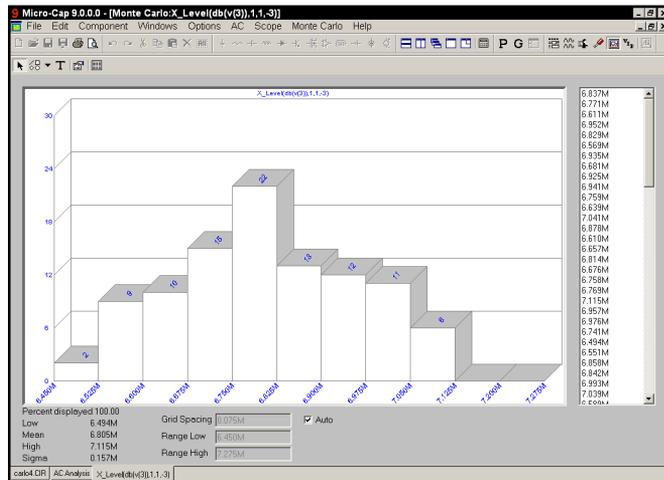
Figure 10-7 AC bandwidth histogram using the X\_Level function
