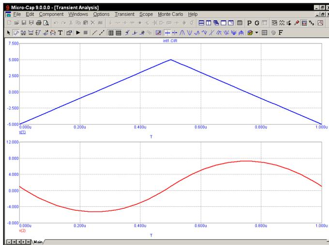
**Figure 11-5 Transient analysis of the circuit**
