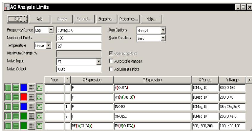
Figure 5-8 The Analysis Limits for Noise plots
