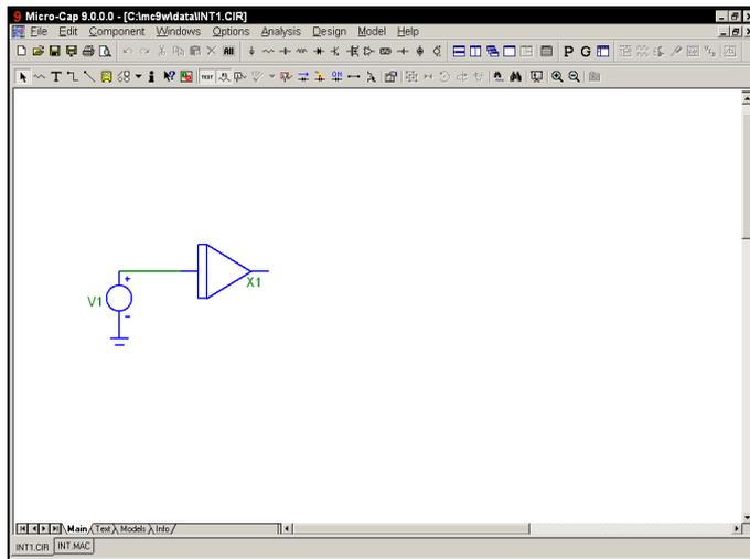
**Figure 11-4 The INT macro used in a circuit**
