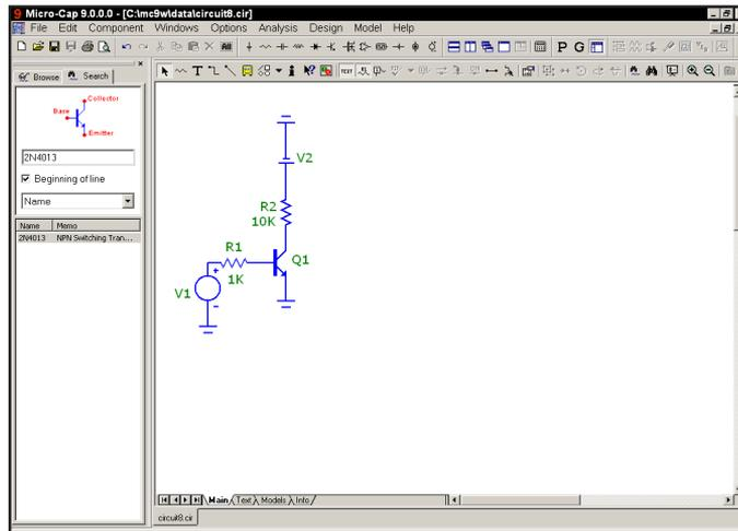
**Figure 3-7 The circuit after adding the bipolar stage**
