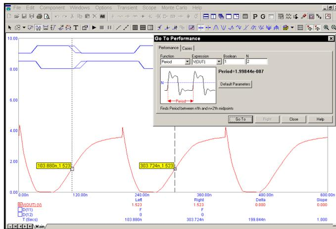
**Figure 7-20 Measuring the pulse period**
