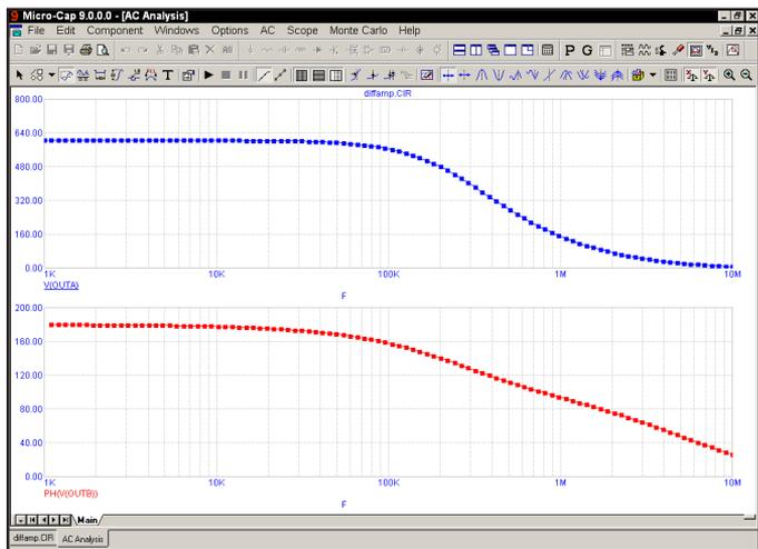
**Figure 5-5 The plot using the log option**
