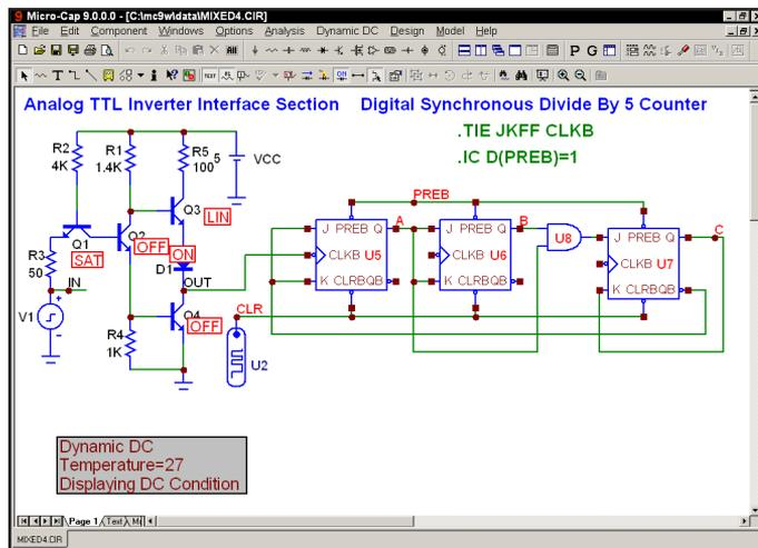
Figure 2-9 Operating point DC conditions
