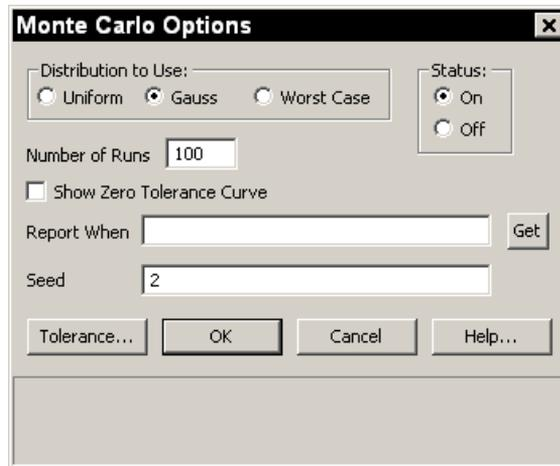
The Monte Carlo options are set to run 100 runs using a Gaussian distribution. A seed of 2 is used. Click on the OK button and press F2 to start the runs. The curves accumulate on the screen and the result looks like this:
