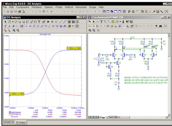
Figure 8-9 DC transfer function plot
