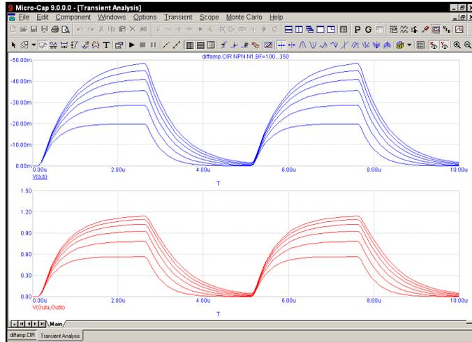
**Figure 9-2 Stepping BF in four transistors simultaneously**
