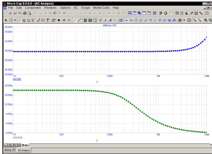
**Figure 5-9 Plots of input and output noise**
