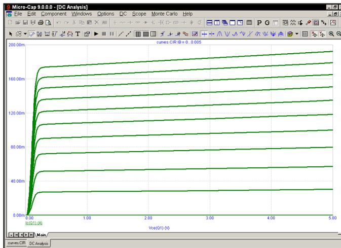
**Figure 6-3 DC analysis plot of IV characteristics**
