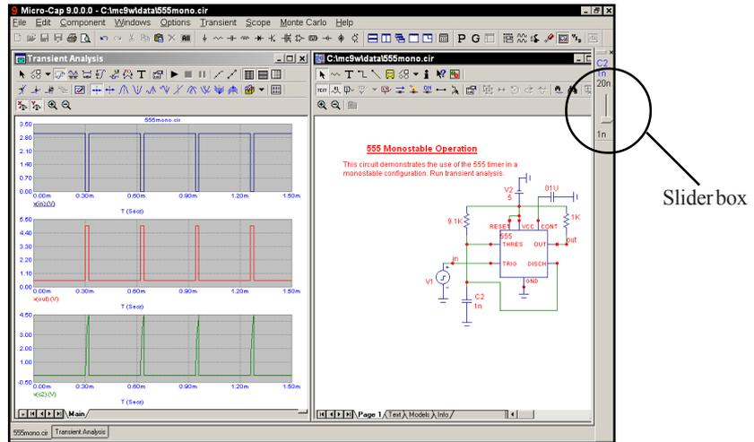
**Figure 4-17 Effect of sliding the C2 value to 1n**
