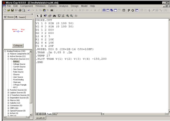
**Figure 3-21 The sample SPICE circuit**
