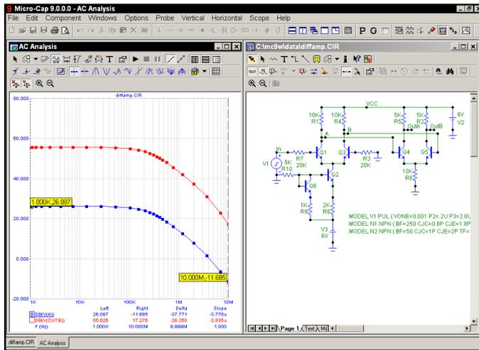
Figure 8-6 Reading AC gains using the Cursor mode
