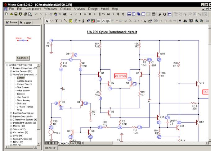
Figure 3-17 The UA709 circuit
