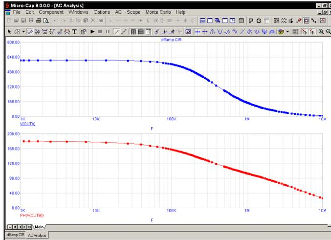
**Figure 5-4** The plot with *Maximum change %* set to 1%
